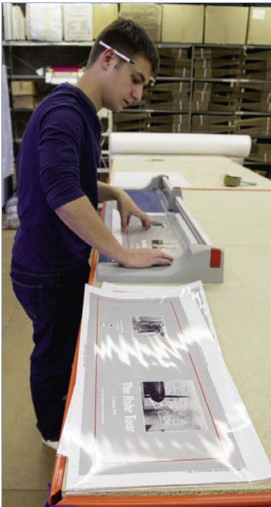
Covers are printed on an Epson inkjet and laminated, before being trimmed.
